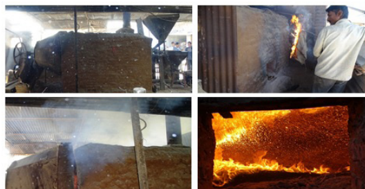
Fig. 12: Open combustion of sawdust in M/s Swastik Poha factory, Umreth, Gujarat
