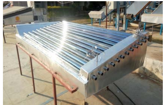
Fig. 6: ETC tube based dryer prototype
