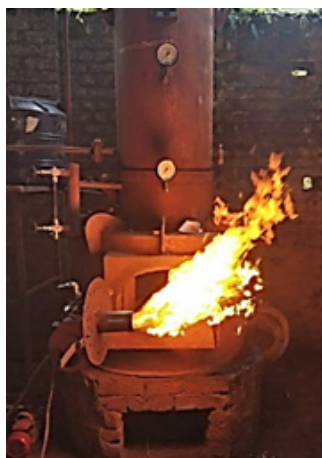
Fig. 18: A bio-oil based burner developed at SPRERI
