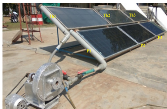
Fig. 1: Solar thermal and PVT collector test set-up
