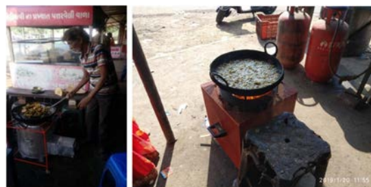
Fig. 19: SPRERI dhabha size forced-draft and natural-draft IBCS
