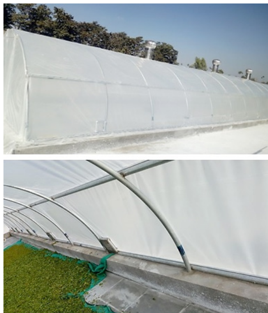
Fig. 26: Walk-in type solar tunnel dryer at M/s Geo-Fresh Organic, Sidhpur
