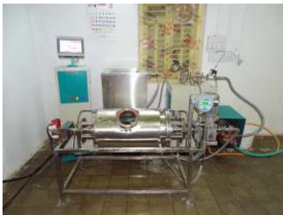
Fig. 6: Solid state fermentor for simultaneous saccharification and fermentation
