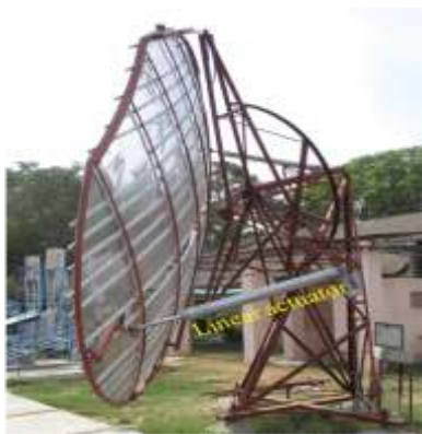
Fig. 4: Linear actuators fitted with the system for semi-automatic tracking
