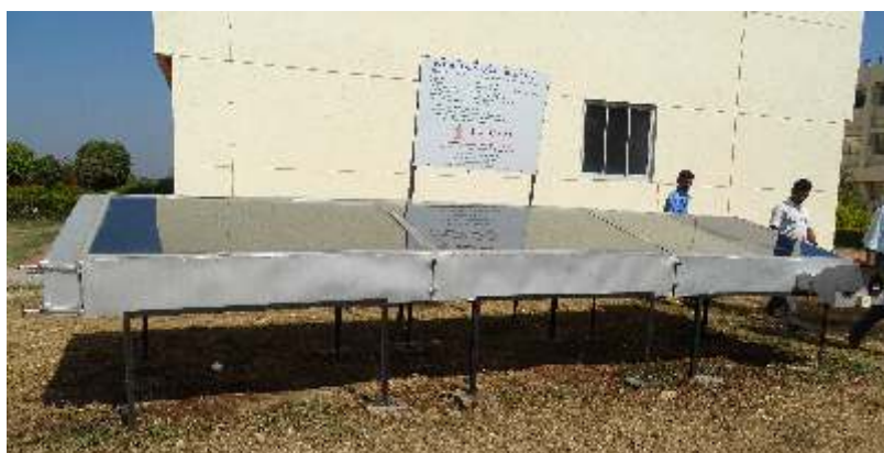
Fig. 25: PV integrated solar tunnel drier installed at Directorate of Medicinal and Aromatic Plants Research, Anand
