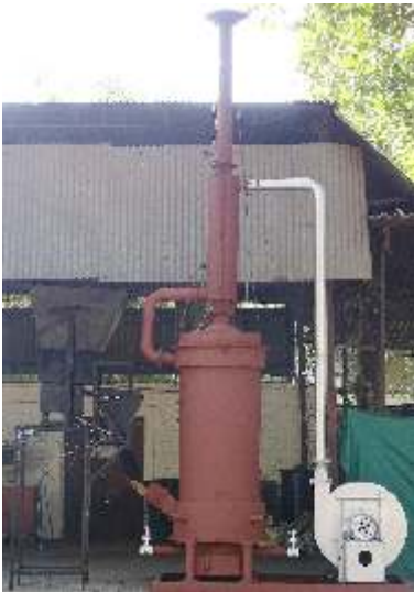
Fig. 13: Photograph of automatic feeder integrated biomass combustor cum hot air generator
