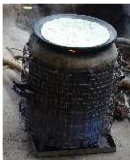
Fig. 22: The SPRERI-TECH improved biomass cook stove in use and the abandoned traditional chulha at Mahelav village
