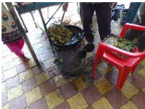
Fig. 20: SPRERI dhaba size, forced-draft biomass cook stove in use at a dhaba
