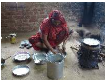
Fig. 22: The SPRERI-TECH improved biomass cook stove in use and the abandoned traditional chulha at Mahelav village
