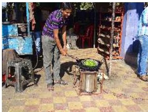
Fig. 20: SPRERI dhaba size, forced-draft biomass cook stove in use at a dhaba
