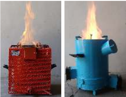
Fig. 12: Images of the SPRERI designed community sized (a) natural-draft and (b) forced-draft cook stoves
