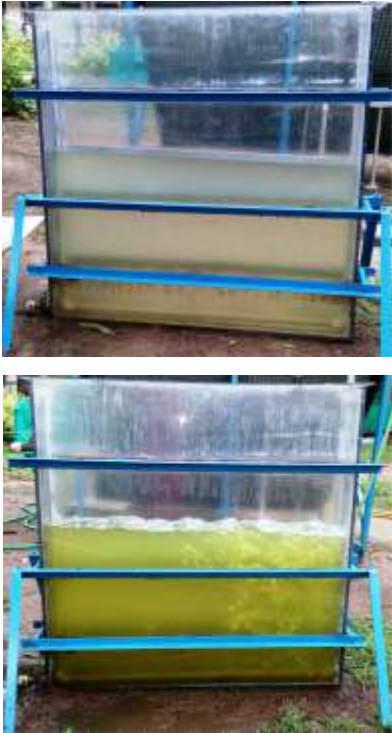
Fig. 7: Microalgae cultivation in out-door flat-plate photo bio-reactor grown in F/2 media. (top) without inoculum on day 1 and (bottom) after 10 d microalgae growth
