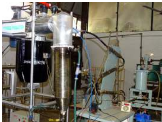
Fig. 10: Experimental set-up for biomass pyrolysis at SPRERI
