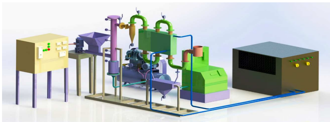
Fig.23 Schematic arrangement of the SPRERITECH fast pyrolysis system
