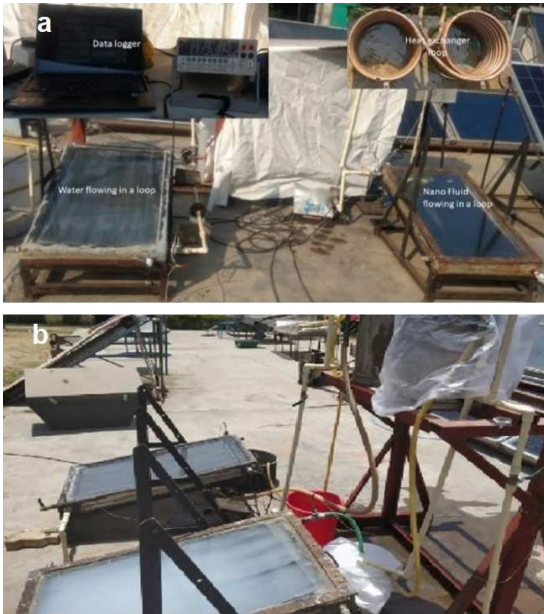
Fig.4 (a) Working of nano-fluid in indirect absorption mode (b) Working of nano-fluid in direct absorption mode
