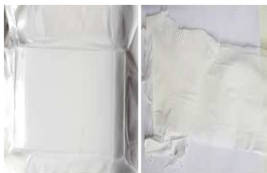
Fig.17 Nano-fibers (a) PVA (12%)-Control; (b) PVA (12%) + protein (20%)
