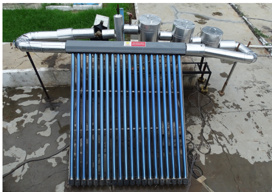
Fig.2: Solar ETC-HP collector with three pressure cooker in series
