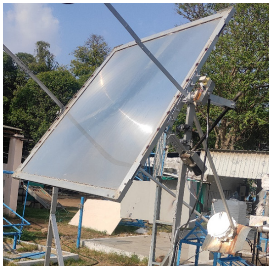
Fig. 1: Fresnel lens integrated with dual-axis tracker and thermal storage device
