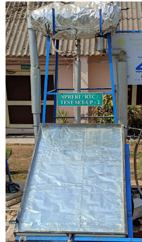
Fig. 9 Direct absorption type solar FPC collector on test bench
