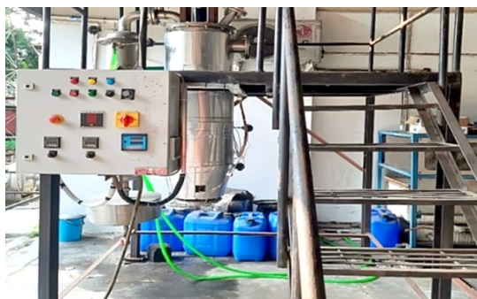
Fig. 27 Image of the installed pilot-scale (5 kg) reactor for the production of activated carbon from bio-char of agro-residues
