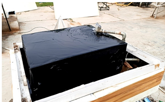
Fig. 7 Arrangement for evaporation area enhancement within the basin
