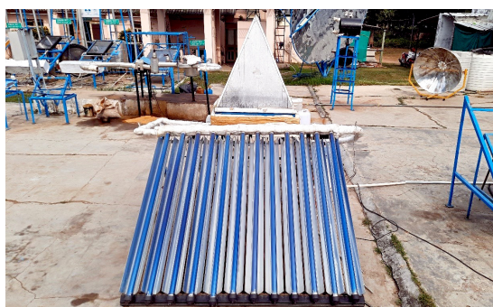
Fig. 8 CPC heat pipe solar still (Prototype-2)
