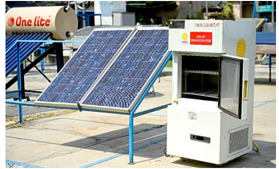
Fig. 12 Front door solar refrigerator with 15 kg ice bank on top
