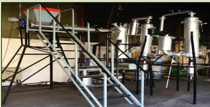
SPRERI-TECH Continuous Torrefaction System: Biomass Processing Capacity ~20 kg/h
