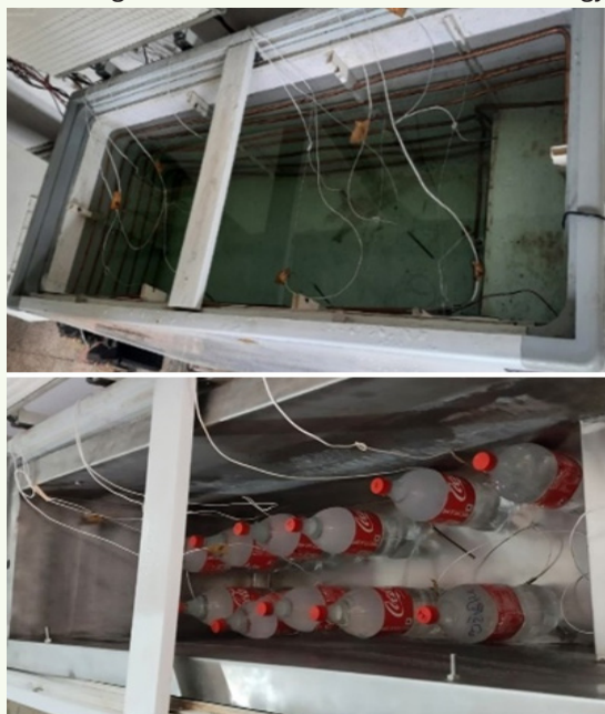
Figure 1.6: Modified refrigerator ( top ) and water as load in chamber ( bottom )
