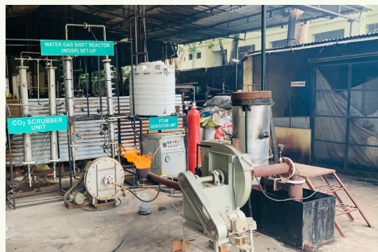
Figure 4.2: WGSR integrated with DDG for hydrogen generation
