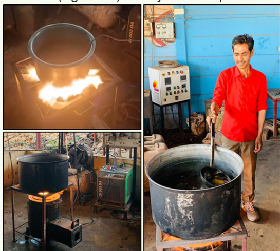
Figure 3.1: Combustion of bio-oil in developed burner at the user site
