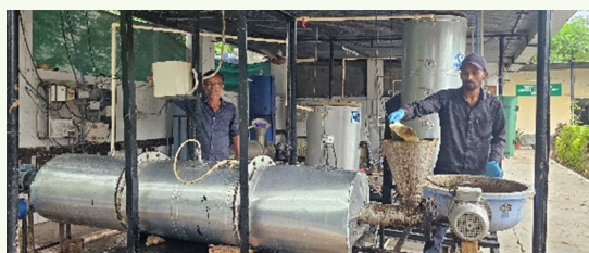
Figure 2.5: Horizontal flow anaerobic digester
