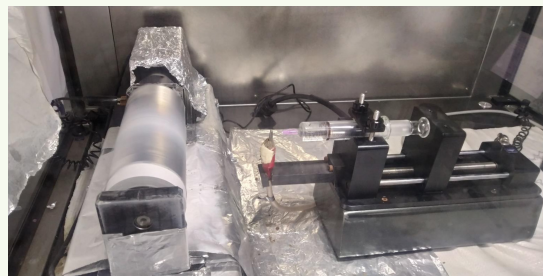
Figure 2.9: Electrospinning equipment for nanocomposite films preparation
