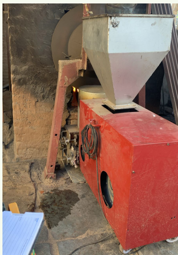
Figure 3.2: Pellet burner integrated with the roaster at the poha-making industry
