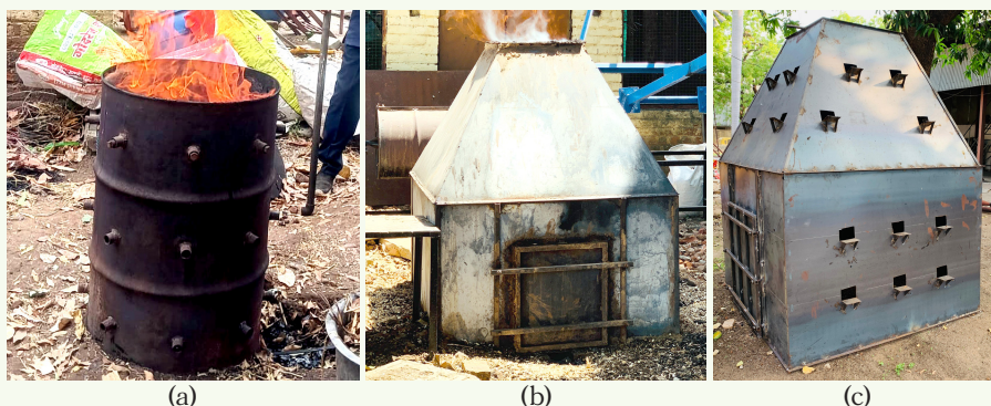
Figure 3.4: Developed vertical biochar kiln (a) 50 kg/batch; (b) 250 kg/batch and (c) 1000 kg/batch
