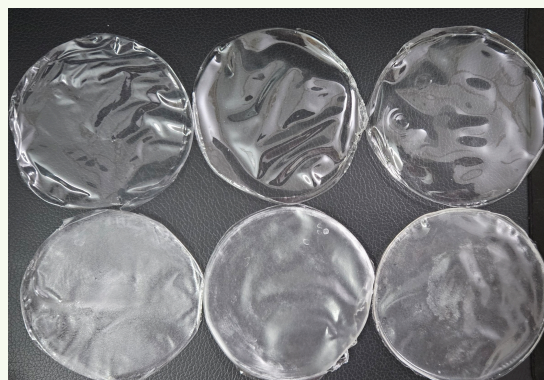
Figure 12: Biocomposites with 0.5% MCC and varying PVA (2.5%, 5%, and 7.5%)
