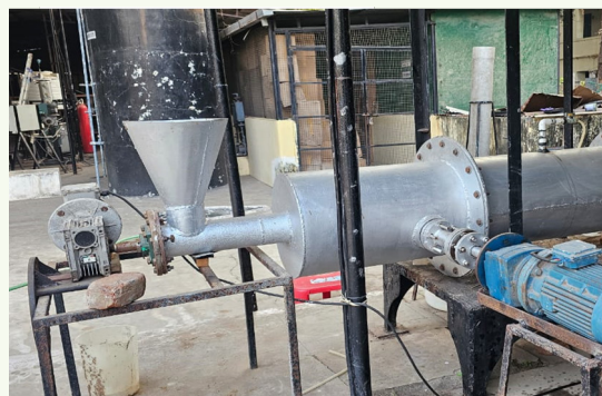
Figure 17: Design of horizontal flow digester and screw feeder (top) and the fabricated digester (bottom)
