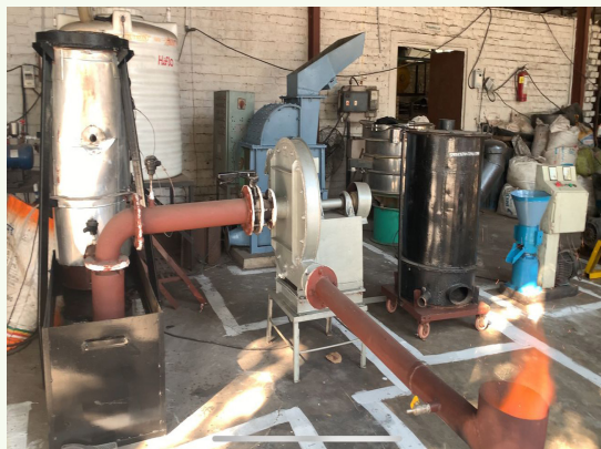
Figure 23: Down-draft gasification system (capacity 15 kg/h) operated on charcoal of babool
