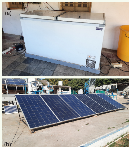
Figure 4: Up-scaled solar refrigerator of 500 L capacity (a) and Solar PV array for power supply to refrigerator (b)
