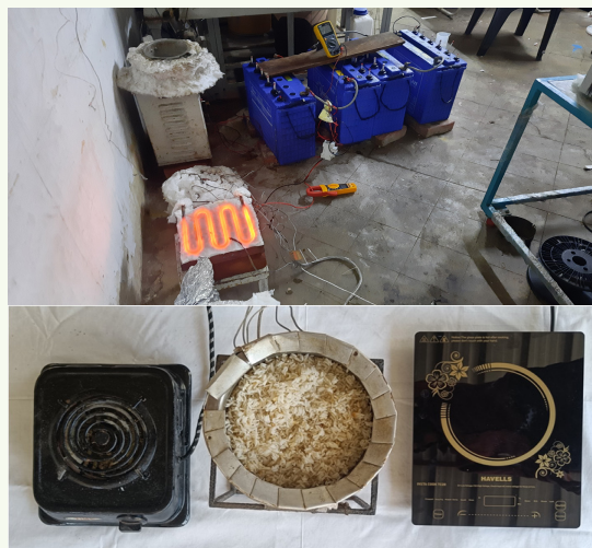
Figure 5: DC heater with TES charging set-up and cooking on induction stove
