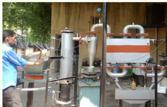
Figure 25: Integrated WGSR and fluidized bed gasifier for enhanced Hydrogen production via biomass gasification
