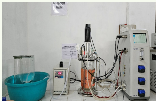
Figure 24: Bio-hydrogen production reactor (5L capacity)
