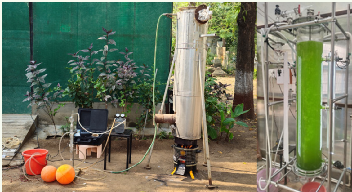
Figure 14: Microalgae experiments for flue gas sequestration
