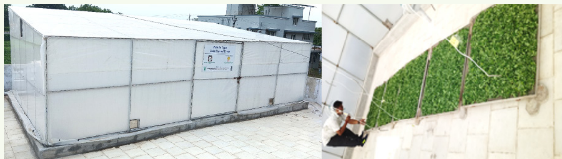
Figure 1: Solar walk-in type dryer installed at M/s CZ Patel & Sons, Boriavi village, Gujarat (left) and Methi leaves loaded in the dryer (right)
