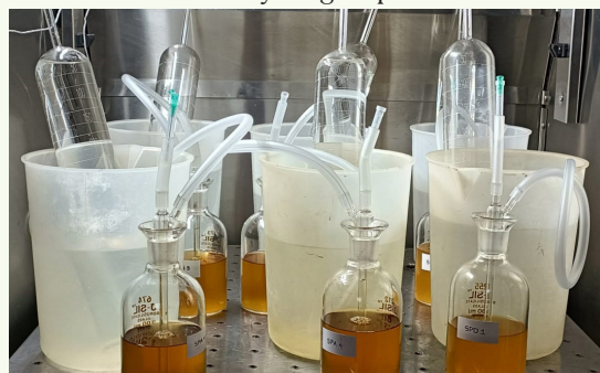
Figure 26: Experimental setup for Biohydrogen production
