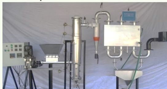
Figure 21: Fluidized bed oxidative fast pyrolysis system for utilization of banana tree waste
