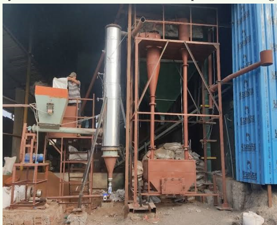
Figure 19: Fluidized bed gasification system installed in Poha making industry
