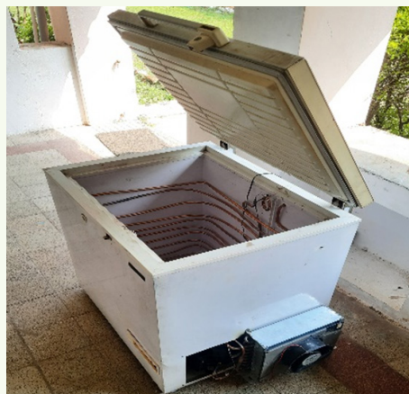
Figure 8: Up-scaled solar DC refrigerator with thermal backup
