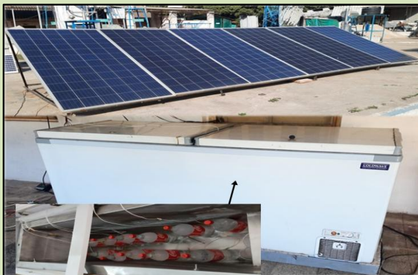
Solar refrigerator with cold thermal energy storage
